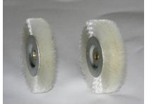
It use saw belt machine to process deciding and judgement in iron industry. For lengthen saw belt service life,installing swarf brush to clear saw blade is the most important thing for saw belt machine.
